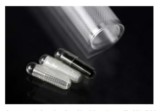
**Figure 1:** Example of microdevice for oral drug delivery. This is a self-unfolding foil that aligns to the intestinal wall (rat or pig). Hereby, we have, among others, achieved oral delivery of insulin [2]
