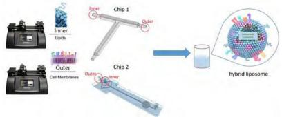
Figure 1: Schematic representation of setup producing hybrid liposome through microfluidics.
