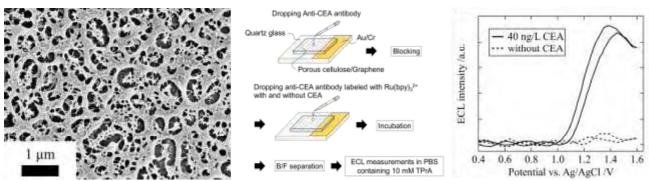
Figure 1: SEM image of porous cellulose. Figure 2: ECL-based immunoassay using cellulose/graphene films.
