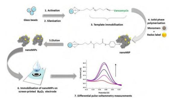
**Figure 1:** General principle for Electroactive Molecularly imprinted polymers Nanoparticles (e- MIP NPs) on SPE
