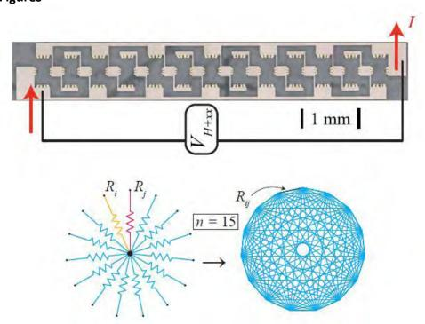
**Figure 1:** (Top) An example 13-element graphene-based array for obtaining quantized resistances other than  $h/2e^2$ . (Bottom) A mathematical star-mesh transformation for a 10 G $\Omega$  quantum electrical standard is illustrated, representing a possible configuration that is within fabrication capacities.
