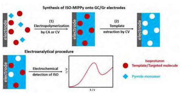
**Figure 1:** Schematic representation of the procedure used for the preparation of ISO-MIPPy films onto exfoliated graphene electrodes, including two steps: 1) electropolymerization of MIPs by CA and/or CV, and 2) the CV extraction of ISO molecules.
