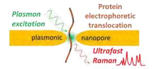
Figure 1: Sketch representing the concept of single molecule identification by means of Raman fingerprint.
