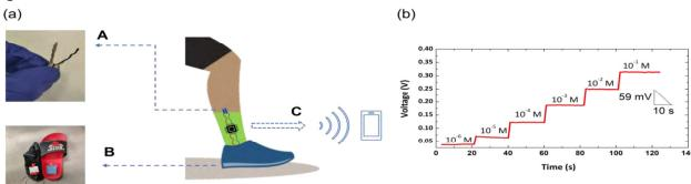
(a)Illustration of self-powered Na $^+$  wearable sensor with (A) conductive ink-coated cotton yarn-based sensing unit, (B) shoe sole based TENG and (C) BLE module. (b) Response obtained when different concentrations of Na $^+$  were added to the sensor.
