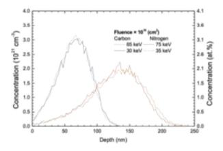
Figure 2: Concentration profiles of Carbon and Nitrogen
