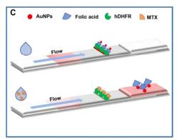
**Figure 1:** Schematic illustrations of the multiplexed paper-based device for the simultaneous detection of three salivary biomarkers (A), doxorubicin POC device (B), and methotrexate (MTX) lateral flow device.
