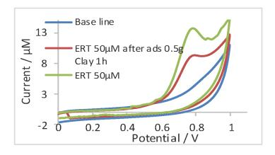
Figure 1: Cyclic voltammetry of ERT before and after the adsorption process on inactivated clay.
