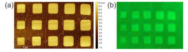
**Figure 1:** (a) AFM height image of Eu-organic film selectively deposited on predefined oxidized graphene patterns. (b) FLIM image of the same area excited by 514 nm laser with 20  $\mu$ W power.
