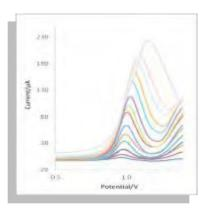
**Figure 1:** Voltammograms of CV (left-E=1.5:-1.5 V) for three types of modified electrode in acetate puffer, pH 5; and Voltammograms of DPV (right- E=1-1.8 V, teq=10 s, scan rate=0.05v/s) for CPE modified with graphene oxide and ZnO, in different concentration of AZI.
