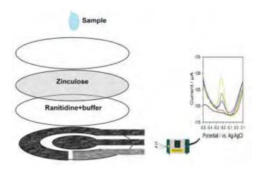
**Figure 1:** Electrochemical paper analytical device for nitrate determination.
