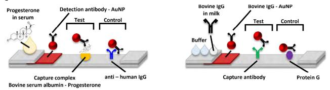
**Figure 1:** Lateral flow assays detection schemes for estrous determination in serum (left) and inflammatory latte mastitis phase detection in milk (right).
