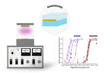
**Figure 1:** Schematic illustration of a nanoband electrode and calibration curves from the macro and nano electrode for DNA sensing
