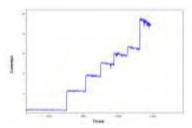
**Figure 1.** The amperogram obtained ate GCE-GrCOONi electrode after injection of the HMF. Operating potential 0.6 V, pH=12 (KCl+NaOH).
