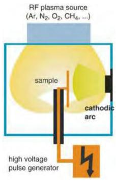
Figure 1: Schematic of the MePIIID deposition system with auxiliary plasma source
