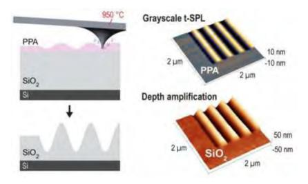
**Figure 1:** Schematics (left) and AFM profiles (right) of t-SPL patterns after writing in PPA and after etch transfer into SiO2. The sinusoidal surface profile can be amplified without shape distortion and without increasing surface roughness.
