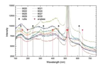
**Figure 4:** Raman spectra of selected samples after implantation, together with reference spectra of a rutile thin film and anatase powder (APS 32 nm, Alfa-Aesar).17 The prominent peak at 520 cm-1 arises from the Si substrate
