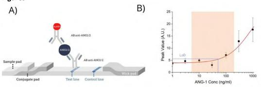
**Figure 1:** A) Representation of the main components and operation of a LFA schematic of the procedure based on immunosandwich recognition, with a positive sample testing B) Final prototype results with their limit of detection and the clinical range of ANG-1 Ab4/Ab7.
