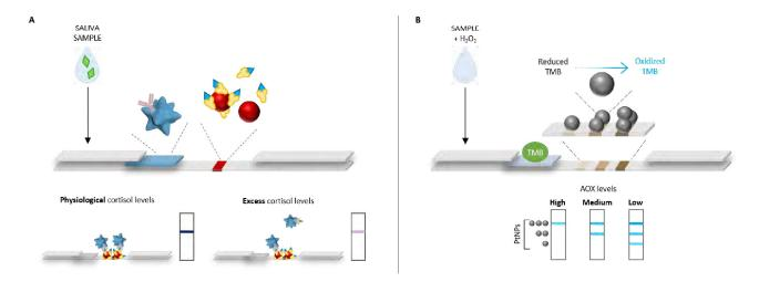
**Figure 1:** Scheme and working principle of the two colorimetric LFDs. (A) competitive dual-color plasmonic immunosensor for salivary cortisol evaluation, providing a blue-to-pink color change of the test line depending on the hormone's levels. (B) competitive multi-line PtNP-based LFD for antioxidants species assessment, providing a number of blue test lines inversely proportional to the antioxidants content of the sample.
