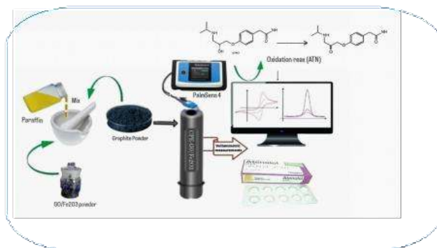
Figure 1: Schematic determination of ATN with Fe 2 O 3 -rGO/CPE sensor
